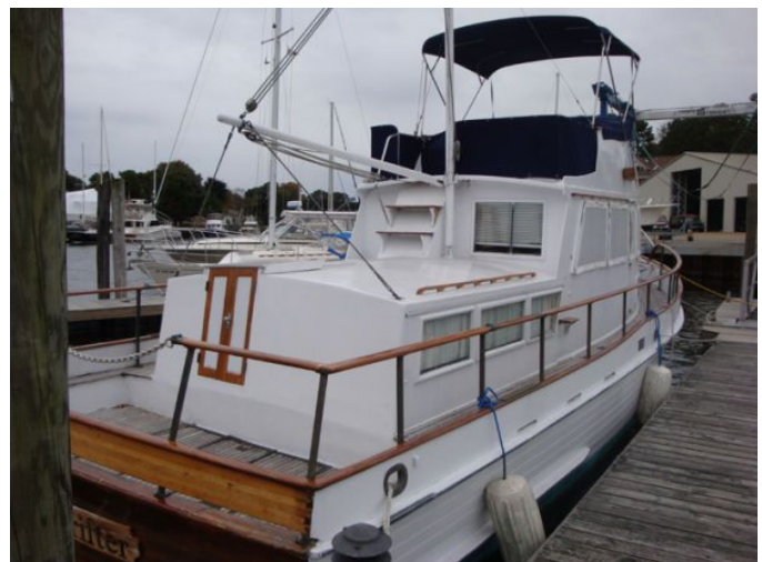
Photo Of The Grand Banks 36' Classic Pilot House, Looking Aft - Note The Limited Rear Visibility.
