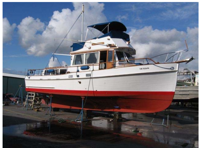
Example Of Deep Keel On A 36' Grand Banks Classic Image Courtesy gbwoodies.com
