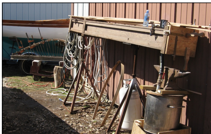
Steam box (foreground) and bending jig (background)
