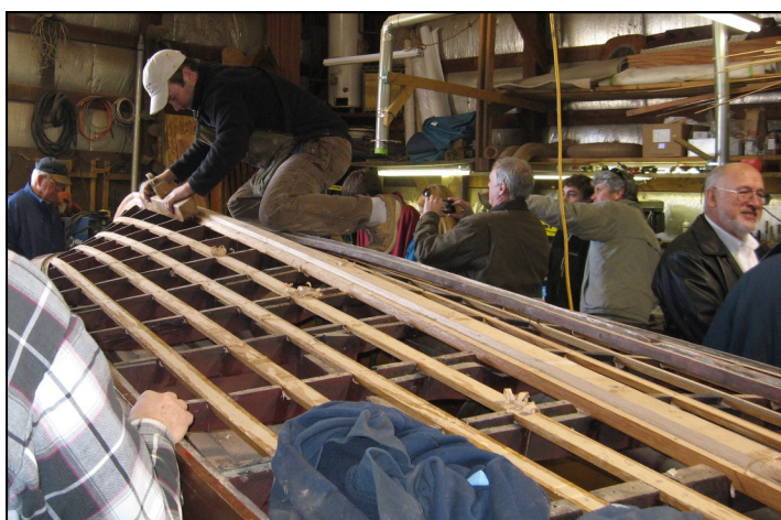
Lars demonstrates fitting a replacement keel
