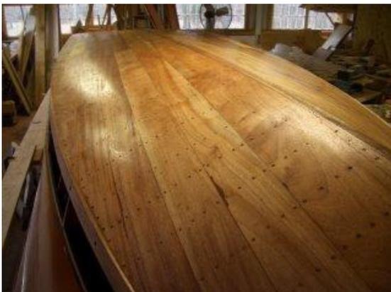
In the photo you will see I cover the bottom with sheet plastic to keep the moisture from drying too quickly (starboard side). The wood does stay stabilized, it won't (or shouldn't leak), this eliminates the wait time for the planks to swell, like yester-year, and best of all the boat will not fall apart.
