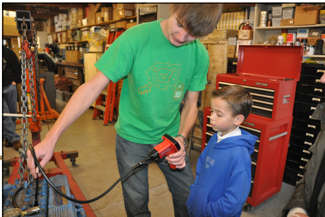
Mitchell O'Day and Alex Svoboda check for stuck valves by inserting a video camera into the engine's cylinders
