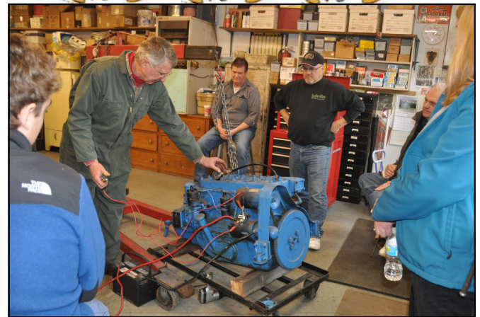
Performing a compression test on the Model K engine
