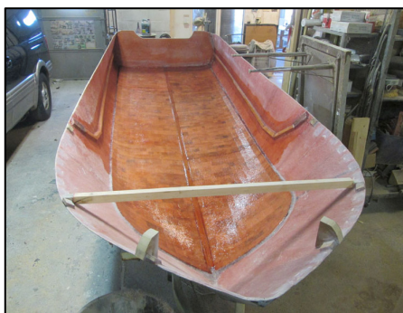
Micolam keel with balsa wood floor
