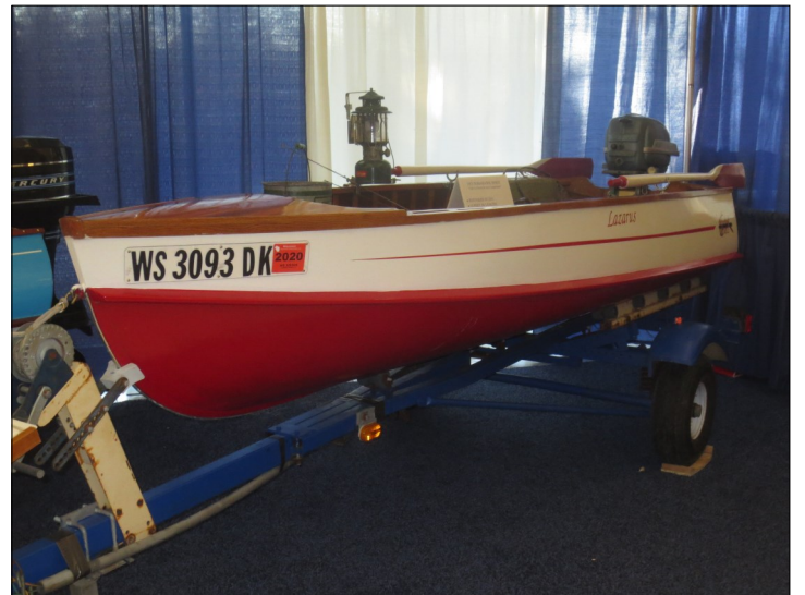
1953 Tomahawk Spirit with the 1953 15 HP Evinrude Super Fastwin. Cedar strip over oak ribs with an optional fiberglass covered bottom, which was then the latest technology in boat construction, sold new for $289.00.
