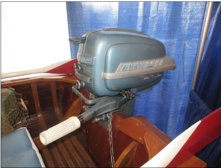
1953 Tomahawk Spirit with the 1953 15 HP Evinrude Super Fastwin. Cedar strip over oak ribs with an optional fiberglass covered bottom, which was then the latest technology in boat construction, sold new for $289.00.
